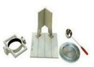
For correct compressive strength of concrete cylinders, the end surfaces of the specimen must be truly flat. If they are not using capping compound and a capper, the faces are plastered flat. Capping set can be used for cylindrical specimen like concrete cylinders of cores. It can be used in laboratory or in field.
