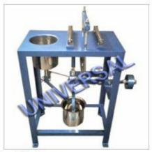
Unit for finding flexural strength of clay roofing tiles and cement concrete flooring tiles.
