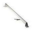
A straight edge approximately 3 meters in length may be used to determine lateral surface regularity of a road surface. This lightweight apparatus is made up of mild steel and is equally supported at both ends producing a set height between the road surface & the beam. Any vertical irregularity is measured using incremented wedges.
