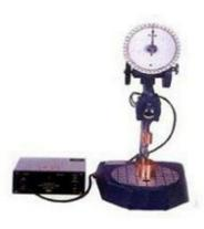
It is used for finding out the rate of hardening of mortars sieved from concrete mixtures, by means of penetration needles of different cross-sectional areas.
