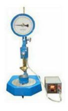
For determining the consistency of masonry mortar.
