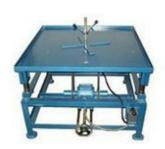
The vibrating table is used for compacting concrete cubes and cylinders.
