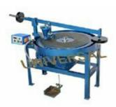
This is used for determination of resistance to wear for cement concrete flooring tiles.
