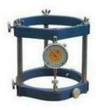
It is designed for finding out the deformation and strains on 15cms. Diameter and 30 cm. High cement concrete cylinders when subjected to compressive loads.
