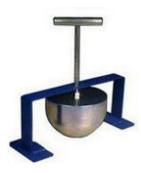
The apparatus is used to determine the workability of Portland cement concrete. The Kelly ball test is considered to be simple and much faster than the slump test. Twice the Kelly ball reading approximately equals the slump.
