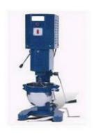
It is used for mixing cement pastes, mortars and pozzolanas.
