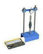
It is used to measure the drying shrinkage of concrete autoclave expansion of port land cement and potential expansive reactivity of cement aggregate combinations in mortar bars during storage, on self drying.
