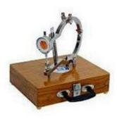
This is for determining the lateral extension of 15cms dia x 30cm high cement concrete cylinders while testing them under compression. Salient Features
