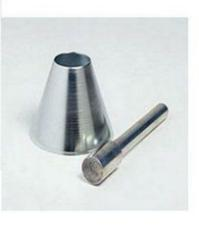
Used for determining the slump of fine aggregate in the determination of bulk and apparent specific gravity and absorption of fine aggregate.
