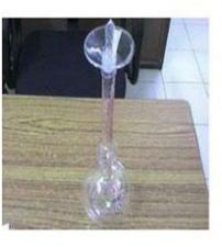
Used for finding specific gravity of hydraulic cement. Made from borosil glass. The flask is 243mm in total height, having a bulb of 90 mm dia of 250ml approximate capacity. The long neck of the flask has at top a funnel of 50mm dia in which fits a ground glass stopper. The neck has over-all 11mm i. D. Upper portion is graduated from 18 ml to 24ml with 0. 1ml graduation. Just at the bottom of the neck 1ml capacity is marked in between there is 17ml capacity bulb.
