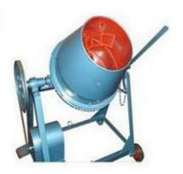
Concrete mixer laboratory type, electrically operated. Designed to remove the burden- some work of hand mixing. Uniform thoroughly mixed batches can be produced. The counter balanced drum is easy to tilt 1. 1/2 to 2cu.ft.mix. The total drum volume is however 3cu.ft. Mounted on a sturdy rubber tyred stand, and the drum is mounted for end discharge and equipped with end towing pole. Equipped with ½H.p. electric motor. Suitable for operation on 220/230 volts A.C. single phase.
