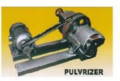
The laboratory pulveriser is a disc type grinder, designed to grind virtually any material to produce a fine mesh sample in one operation. The instrument is useful for assaying, mining and for metallurgical, quarrying, aggregate processing, chemical, geological and industrial laboratories. It is a self contained grinder, with a rotary disc, having a planetary movement in a vertical plane. This feature gives added life to the moving parts and produces a sample of uniform fineness.
