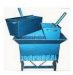
Used for sampling aggregates ores refr actory materials, pigments powdered coal, soap, cement etc.
